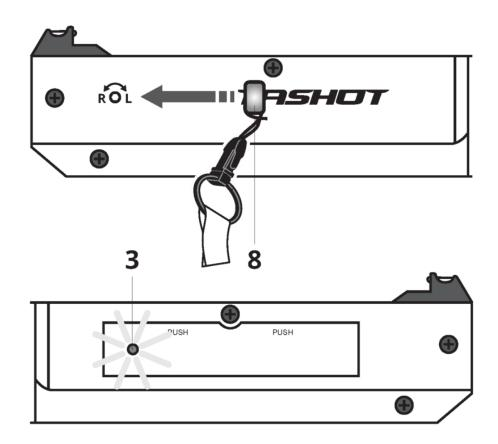
After the battery test, the LED light remains constantly blue to indicate the laser is on and ready for use.
