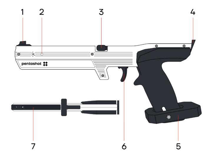
1 — Bead (front sights) integrated into the battery cover
