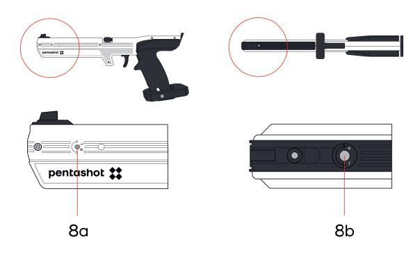
IMPORTANT: The adjustment screw movements must be very small. One turn of an adjustment screw moves the laser dot about 20 cm at a distance of 10 m.
