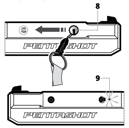
After the battery test, the LED light remains constantly blue to indicate the laser is on and ready for use.
