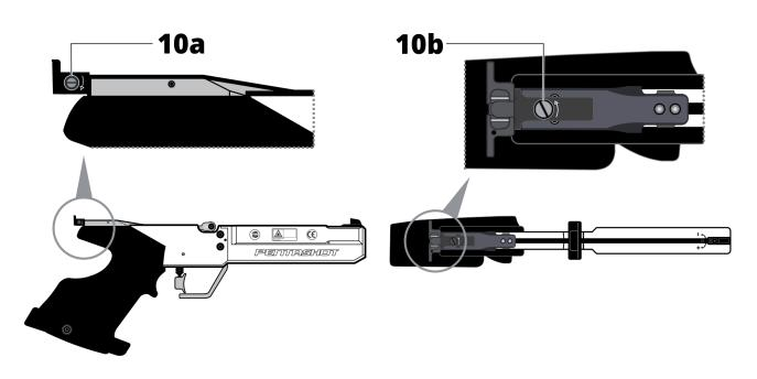
**IMPORTANT**: The movement of the adjusting screws must be very small.
